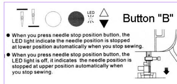
**mod. HQ-1200E with needle position control buttons**
